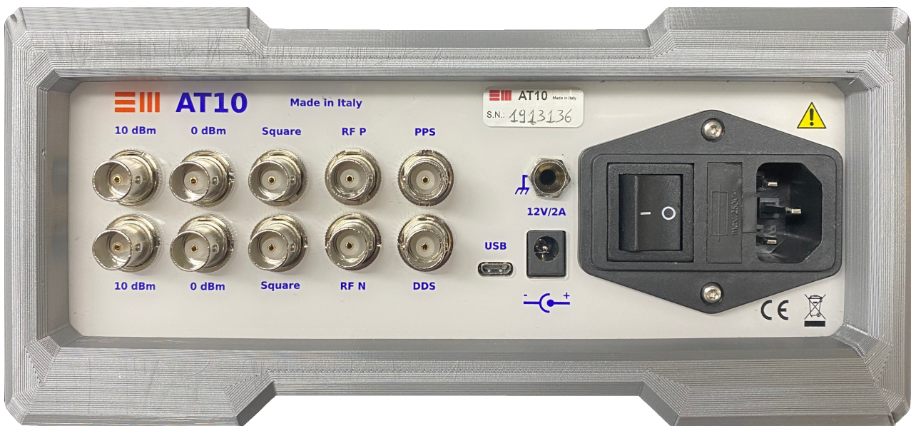
Figure 4: AT10 Rear Panel
